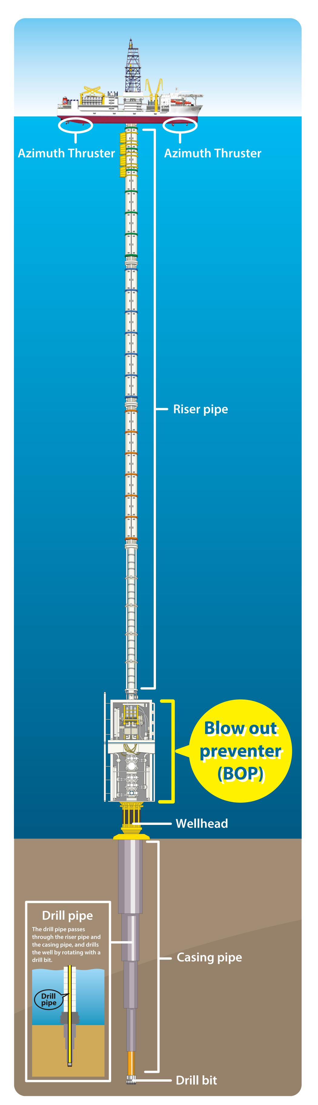
Blow out preventer is installed to the seabed to prevent a blowout of high pressure oil or gas from stratum. In case of a blowout, BOP can seal or shut off a borehole with special valves, one of that can shear even the drill pipe.
