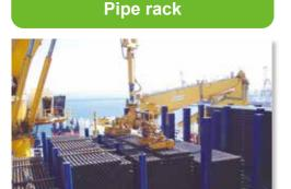
Pipe racks (fore & aft) store drill pipes (each joint ca. 9.5 m) and casing pipes. 10,000 m of drill pipes can be stored. Other tools and equipments for downhole can be stored here as well.
