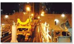
The riser pipe transfer system (RTS) helps move riser pipes to and from the rig floor, and it can be used to move other heavy objects to the rigfloor as well.
