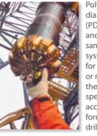
Poly-crystalline diamond compact (PDC) core bit drills and trims core samples. The coring systems are designed for differing sediment or rock hardness, and the PDC bits are also specifically designed according to the formation being
