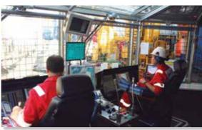
The driller's house ("Dog House") is where all drilling and downhole operations are controlled and monitored. A modern digital system assists the drillers in manipulating all tools and equipment on the drill floor, and monitors downhole conditions in realtime. The BOP control system are also controlled and monitored from here.
