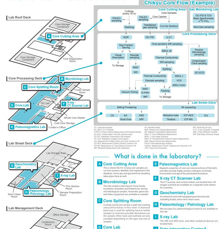
This multipurpose space is designed for the efficient examination, description, and sampling of split core sections. Special facilities Individual working desks and several working
