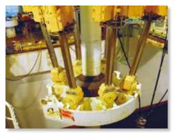
Special hydraulic pistons to secure the riser pipe to Chikyu, which also can apply slack or tension on the riser pipe, as needed. They help neutralize some of the heave from Chikyu's motion in the ocean while drilling under DPS.
