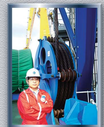
Dead line anchor for fixing the cable. Cable load (weight) is detected by measuring tension at this position.
