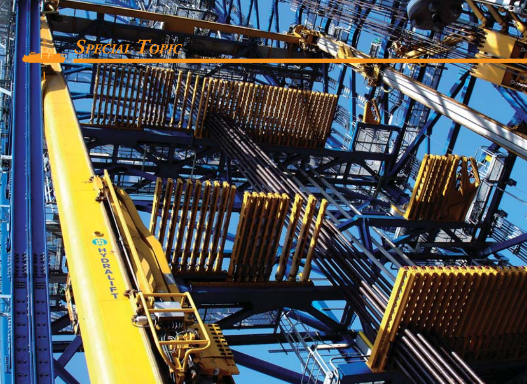
Four drill pipes each of which is 9.5 m long are connected to make a drill pipe of 38 m, and the assembled drill pipes are rested against the Finger Board inside the derrick one after another.
