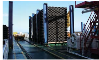
In this cruise, drill pipes of a total length of about 10,000 m were loaded in the pipe rack area.
