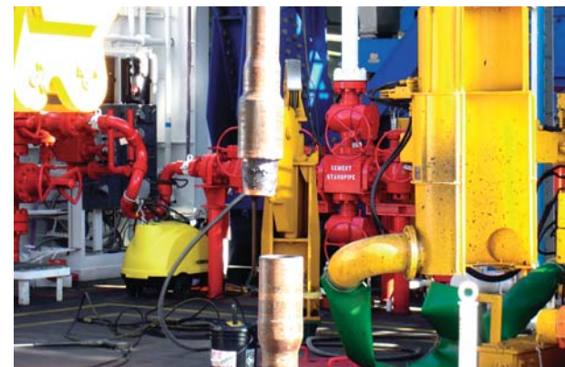
Joined portion of pipes. All the tasks such as position setting and rotating to fasten the joint are automated.
