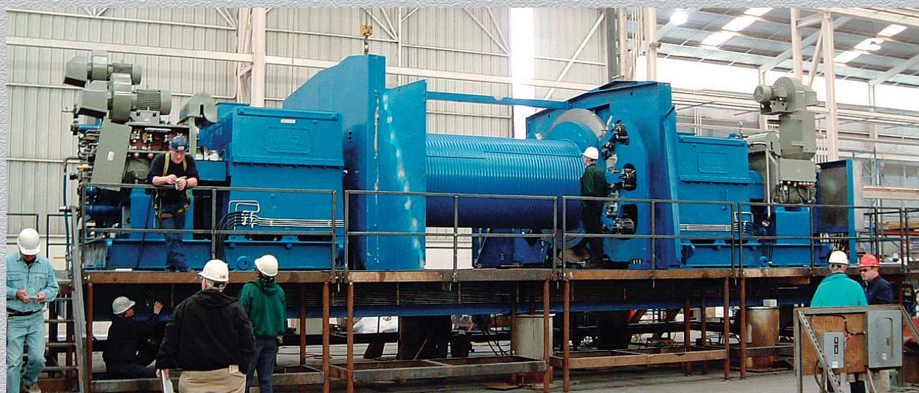
The world's largest drawworks being assembled at the factory in the USA before being mounted on D/V CHIKYU . This photo shows the Draw Works after installation, so the complete assembly cannot be seen.
