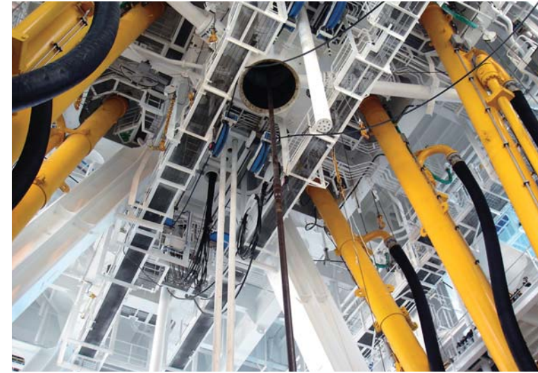
The photo on the left shows the view you can get when looking up from the upper deck under the drill floor. The joined drill pipes are being lifted down gradually, being held by the power slip (black round portion at the center). The photo on the right shows the Moonpool that is the 12 x 22 m opening at the bottom of the drill floor. Pipes are lowered through the Moonpool into the sea.
