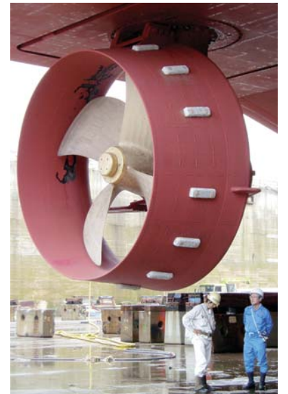
Six Azimuth Thrusters (photo) work to keep the position and direction of the D/V CHIKYU during DPS operations.
