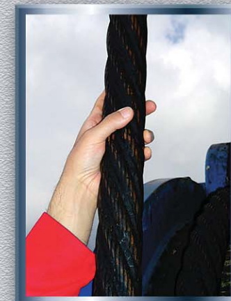
The wire cable is very thick, measuring 54 mm in thickness - almost the same size as a human wrist.
