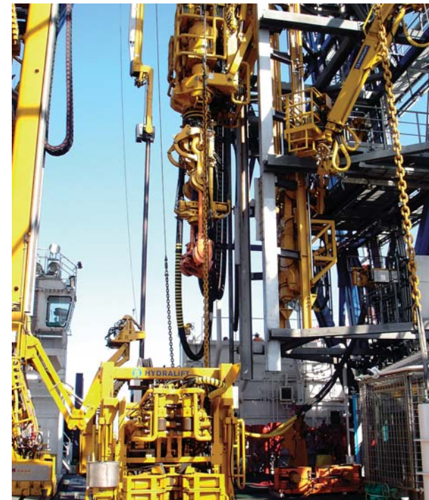
The drill pipes transferred to the drill floor are lifted and connected in a standing position. The machine shown in the lower part of the photo is the Hydraulic Roughneck for joining drill pipes, and the suspended machine shown in the center is the Top Drive for rotating drill pipes.
