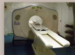
The X-ray CT Scanner examines the internal structure of the core section nondestructively.
