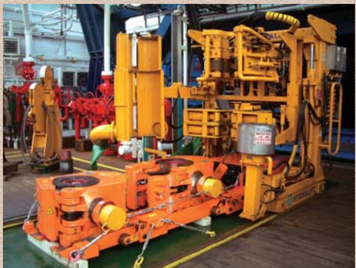
The iron roughneck used for connecting drill pipe sections to the drill string. There are different manipulator arms that can be used on the iron roughneck drill pipe or casing pipe sections with different diameters.
