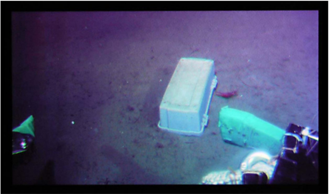
Photograph 9: Image of on-board display screen taken by a digital camera Length of the object: approximately 40cm Right: sample basket of HYPER DOLPHIN (North Latitude: 34.31 East Longitude:139.49 Water Depth 1,841m)
