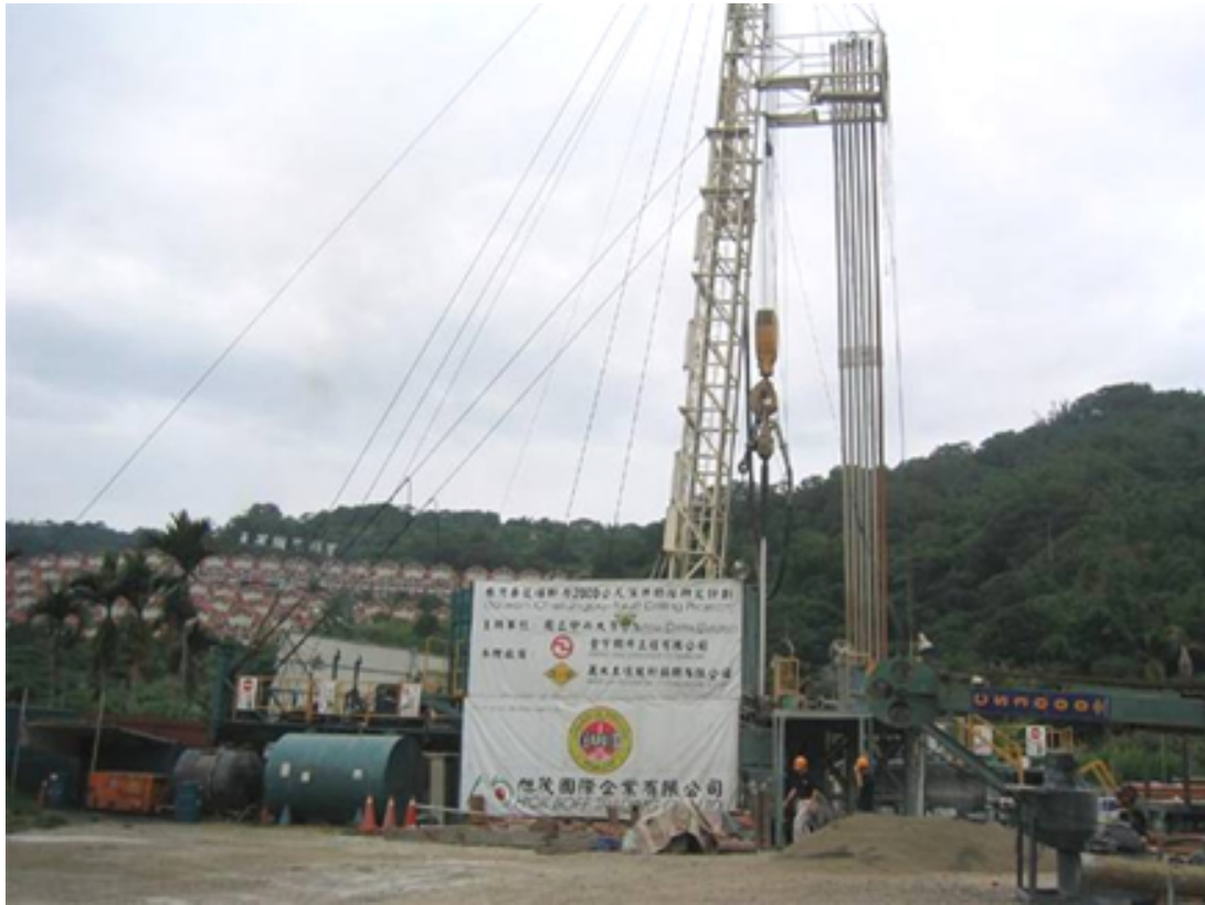
Fig.1 Drilling operation of the Chelungpu fault
