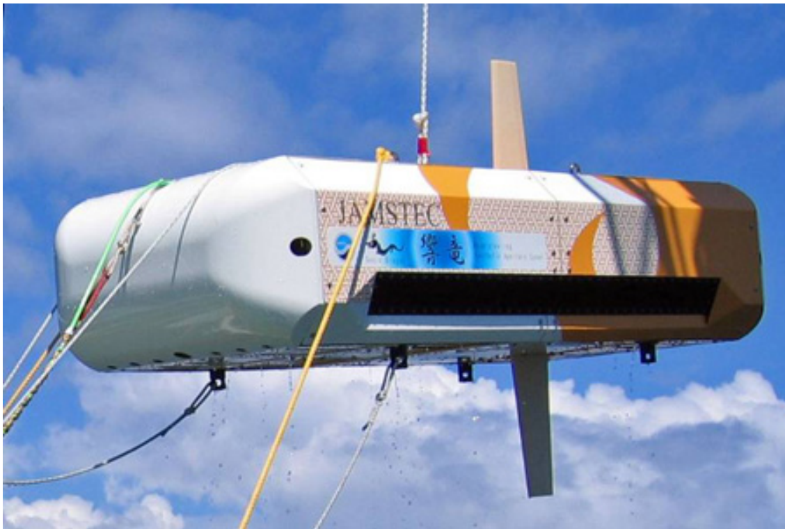
Figure 1: Neutral buoyancy towed vehicle Width: 2.3 m, Depth: 1.2m, Air weight: 100kg
