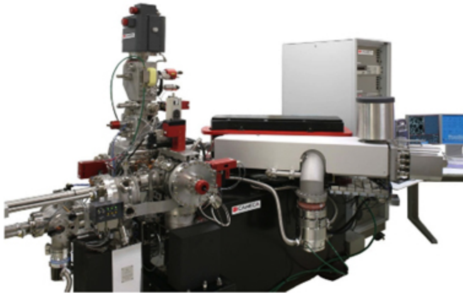
Figure 1. High Spatial Resolution Nanometer Secondary Ion Mass Spectrometry(NanoSIMS)
