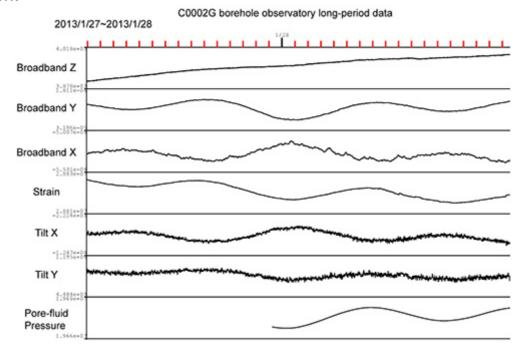
Figure 1 Long-period data (2013/1/27–2013/1/28) from the broadband seismometer (Broadband X,Y,Z), strain meter (Strain), tilt meter (Tilt X,Y) and pore-fluid pressure meter (Pore-fluid pressure) of the long-term borehole observatory connected to the DONET. The effect of tides on crustal deformation is observed.
