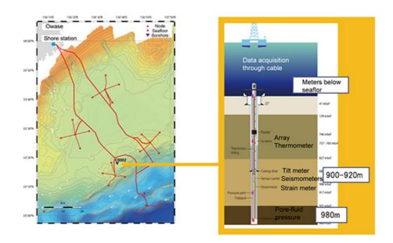
Figure 2 Map of locations of the DONET submarine cable network and long-term borehole observatory and diagram of the layout of sensors in the long-term borehole observatory. The long-term borehole observatory is installed at Site C2 on the map
