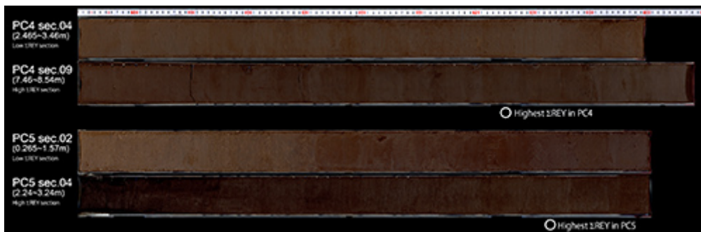
Figure 3. Sediment cores collected at points PC4 and PC5 shown in Figure 2. Sec.04 of PC4 and sec.02 of PC5 are dark brown clay with low concentrations of REY. Sec.09 of PC4 and sec.04 of PC5 are blackish brown clay with high concentrations of REY. O in Figure 4 mark the layers where the concentrations of REY are highest in each core.
