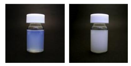
Figure 4. Comparison of a highly translucent nanoemulsion produced by MAGIQ (left) and a conventional emulsion containing micrometer-sized oil droplets (right).
