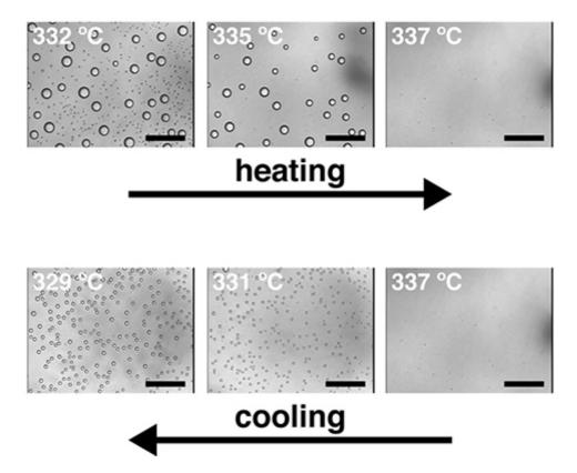
Figure 2. A series of optical microscopic images illustrating the concept of MAGIQ. Scale bars represent 0.1 mm.
