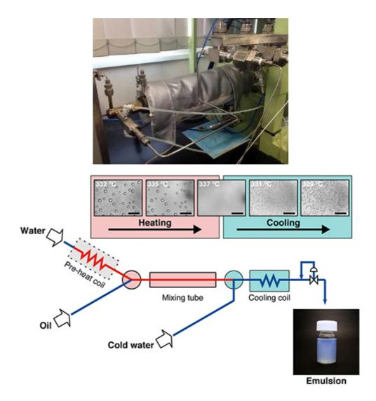
Figure 3. Photograph and schematic representation of a flow-type instrument to perform MAGIQ.
