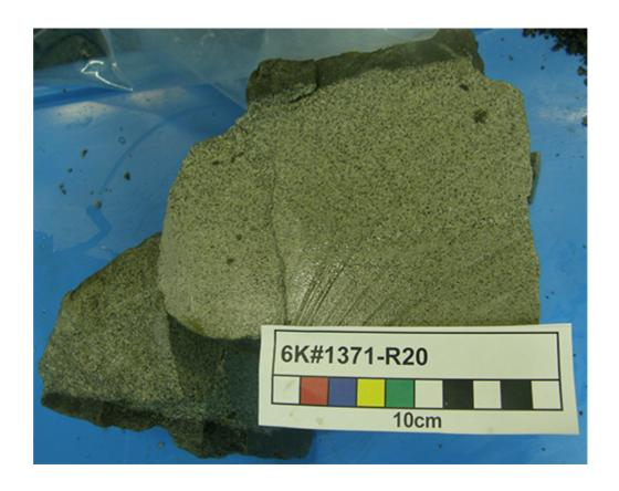
Figure 11. Sandstones sampled at a depth of 6,150m. It is including a quartz.
