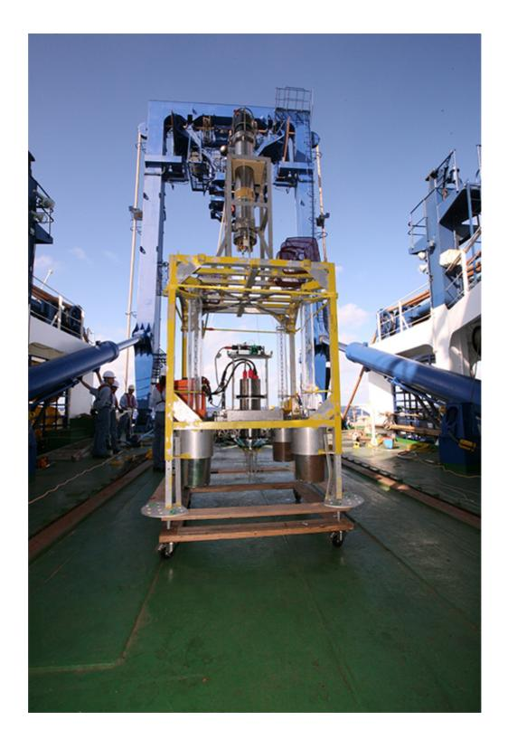
Figure 3. A sediment profiling lander. After the instrument has landed at the seafloor the central titanium cylinder move 20 cm into the seabed in small steps of 250  $\mu$ m. At each step the  $O_2$  concentration is recorded and thereby the oxygen distribution in the sediment is recorded. From the data the scientist can caculate how much oxygen the seabed is consuming and how much organic material that is degraded in the seabed.
