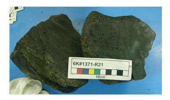
Figure 10. Basalt rocks sampled at a depth of 6,088m. Foaming can be seen.
