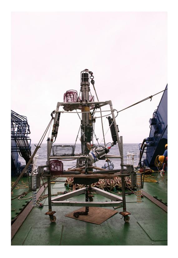
Figure 2. JAMSTEC's free-fall sediment sampling lander system with video camera attatchment. For these surveys, it was equipped with water samplers and a CTD instrument.
