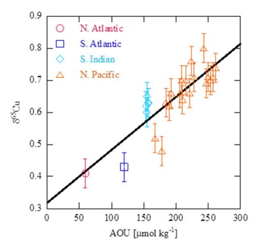
Figure 3:  $\delta^{65}$ Cu vs. AOU for deep seawater. Isotopic ratios shown as  $\delta^{65}$ Cu values become higher in order of that from the North Atlantic to the South Indian Ocean and then the North Pacific, which shows a stronger correlation with AOU.
