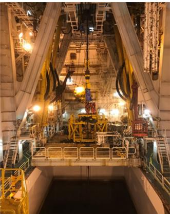
Photo 2 & 3 Preparation for installing wellhead assembly (CORK head) LTBMS sensors are inserted into a drilled hole. After fixing them with cements, the wellhead assembly is installed on the top of the borehole. By connecting submarine cables with the well head assembly, then real-time monitoring of observational data will become available later.
