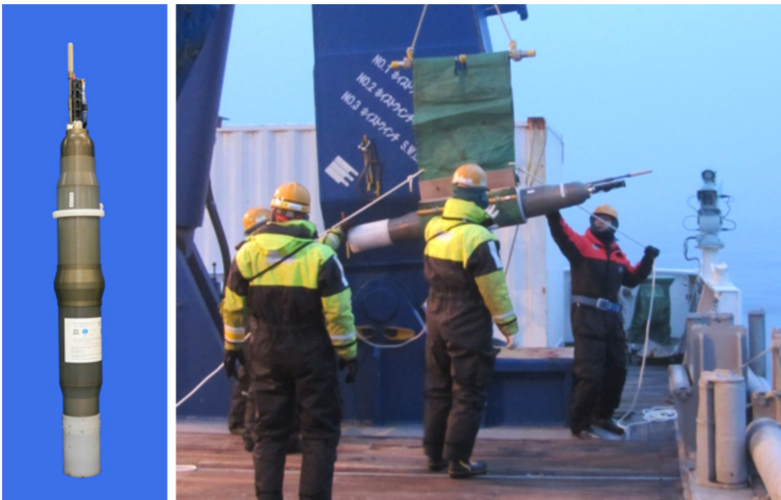
Figure 1. Deep-ocean profiling float "Deep NINJA" is deployed in the Antarctic Ocean from the R/V Mirai .
