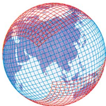
Fig. 1 Yin-Yang grid system.
