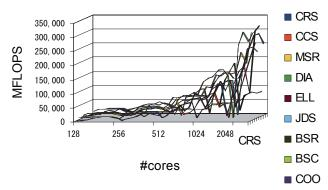
Fig. 6 Performance of spmvtest1 on the Fujitsu PRIMEQUEST Cluster at Kyushu University.
