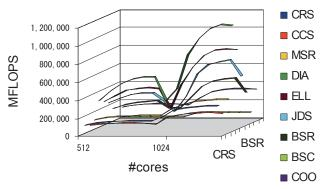
Fig. 7 Performance of spmvtest1 on the Hitachi SR16000 Cluster at Kyushu University.
