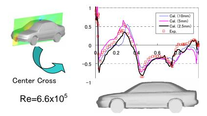
Fig. 4 Comparison of pressure distributions at center cross section of vehicles
