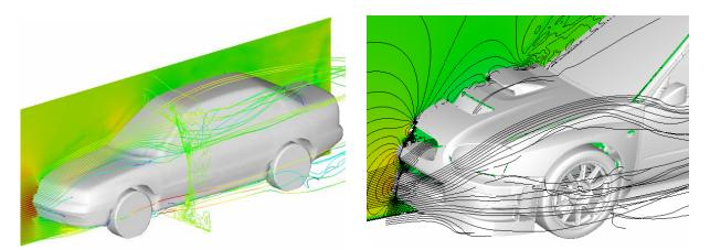
Fig. 5 Analysis result: Flow of the entire vehicle Fig. 6 Analysis result: Flow around the front part of the vehicle
